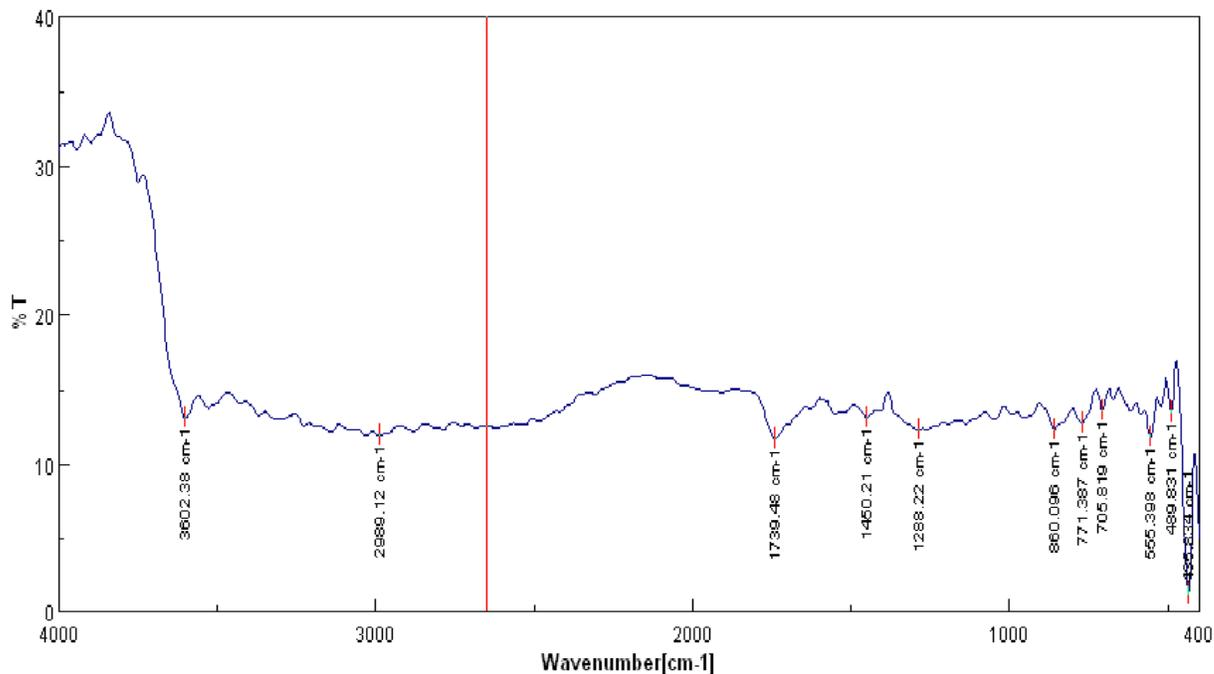
Fig.3 FTIR spectra of DRC(C)
